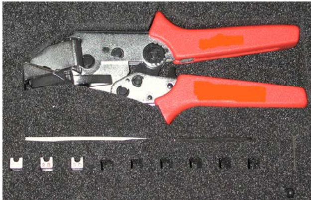
Figure 1B: Access Tool A2 in Case with 2.5mm, 2.8mm, and 3.0mm Inserts.
