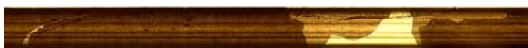
Figure 6D: A Section of Fiber with Secondary Coating Almost Entirely Removed by Tool C.
