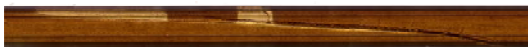
Figure 6C: Fiber Damage along a Substantial Length of an Orange Fiber from Tube C Accessed with Tool C.
