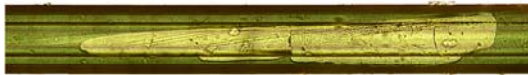
Figure 6B: Fiber Damage on a Green Fiber from Tube C Accessed with Tool C.
